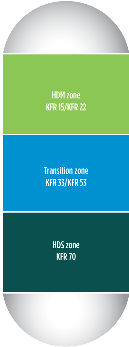
FIG. 4. Albemarle has identified three main reactor zones for hydrotreating residue feedstocks.
