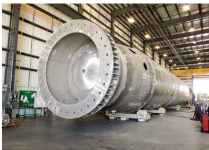
FIG. 1. A large coil-wound heat exchanger in production at Air Products' new manufacturing facility.
