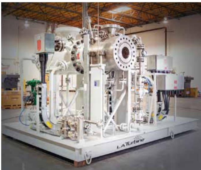
FIG. 1. L.A. Turbine's newest L3000 AMB turboexpander-compressor is scheduled for a 2017 delivery to an African gas processing plant.
