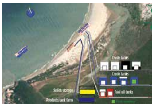
FIG. 4. A refinery model can estimate the number of receiving crude tanks and product tanks, and the storage capacity needed for solids and other products from the refinery.
