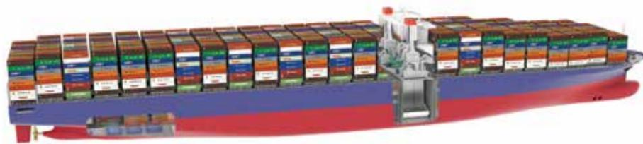
**FIG. 3.** Phase 2 of the PERFECT ship project investigates the possibility of using a combined gas and steam turbine system (COGAS) to power a ULCS. Source: DNV GL.
