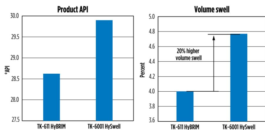
FIG. 3. Obtained volume swell with HyBRIM and HySwell catalysts in hydrocracker pretreatment service.
