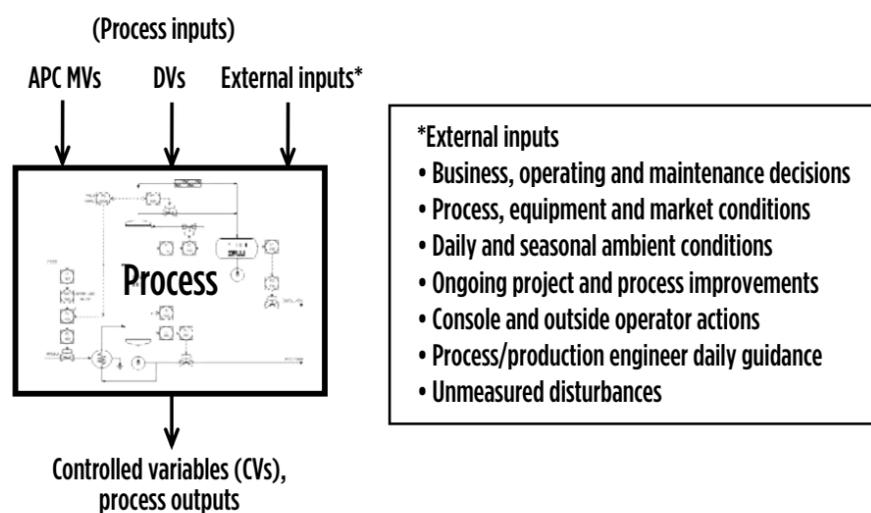
FIG. 2. Many factors affect a process' controlled variables (CVs), making it problematic to identify the particular contribution of APC to benefits or performance.
