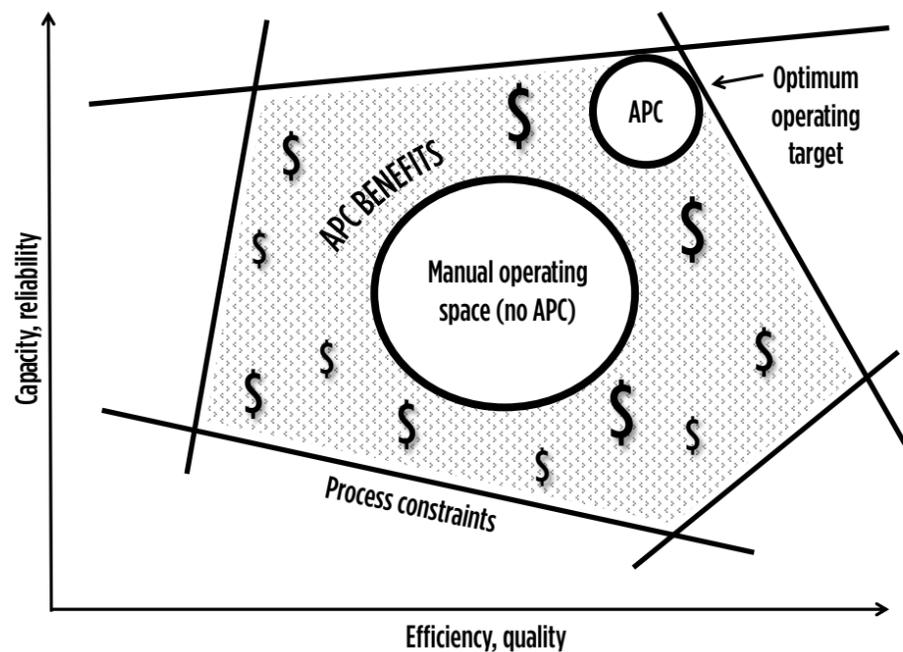
FIG. 1. APC earns benefits by holding the process closer to constraints than manual control, even as the process operating point and constraint limits move dynamically.
