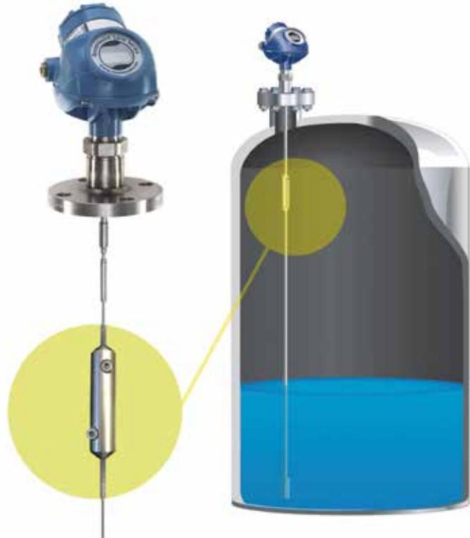
**FIG. 1.** A verification reflector placed on a GWR probe allows for proof testing a high level point without raising liquid levels to that point.
